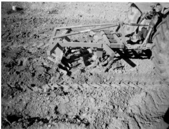
Figure 2. The rotary harrow fabricated for soil loosening
