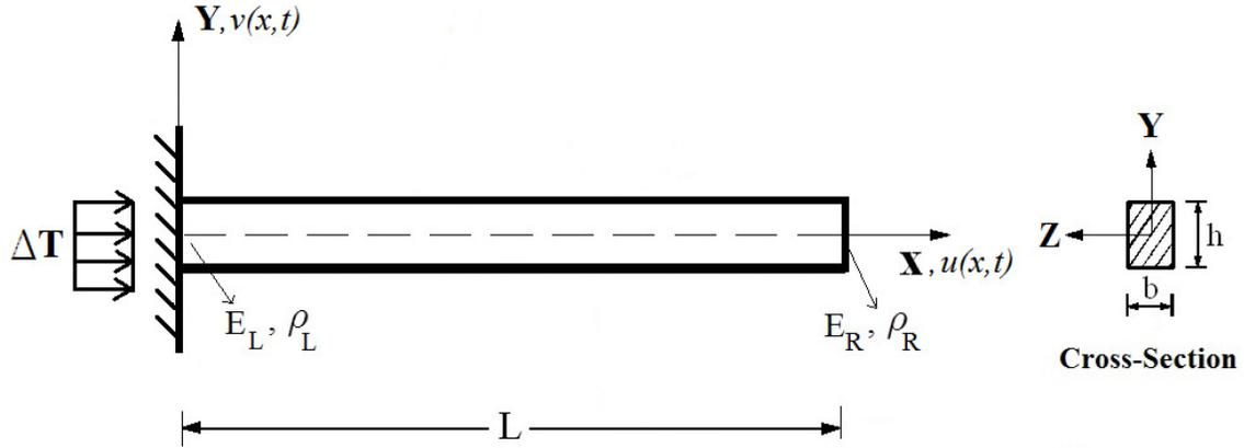
**Fig. 1** A cantilever axially functionally graded (AFG) beam under uniform temperature rising  $\Delta T$ .
