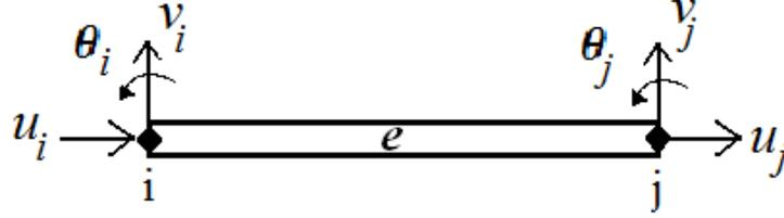
**Figure 2.** A two-node beam element.
