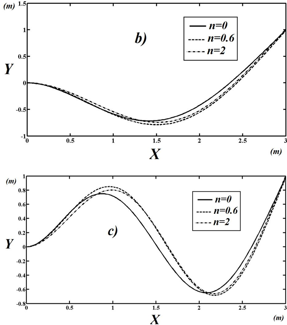
**Figure 5.** The effect material distributions ( $n$ ) on the first three lower vibration modes for Temperature  $T=400$  K. a) First mode shape, b) Second mode shape and c) Third mode shape.
