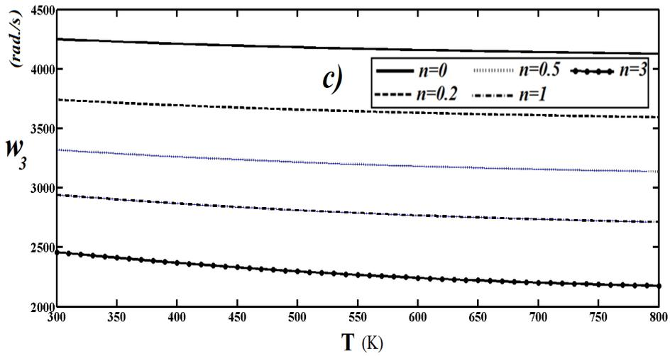
**Figure 3.** The effect of Temperature ( $T$ ) on the first three lower natural frequencies  $w$  for different the material distributions  $n$ . a) First natural frequency ( $w_1$ ), b) Second natural frequency ( $w_2$ ) and c) Third natural frequency ( $w_3$ ).
