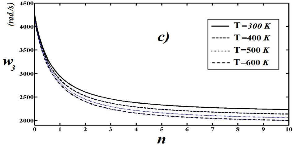
**Figure 4.** The effect material distributions ( $n$ ) on the first three lower natural frequencies  $w$  for different the Temperature ( $T$ ). a) First natural frequency ( $w_1$ ), b) Second natural frequency ( $w_2$ ) and c) Third natural frequency ( $w_3$ ).
