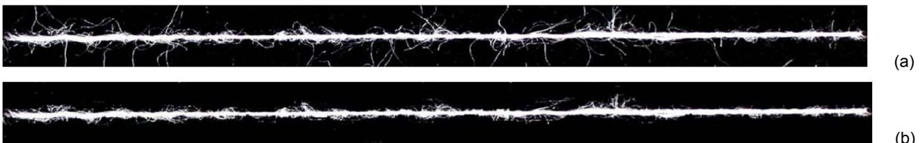
Figure 1. Images of yarn samples (a) before and (b) after image analysis
