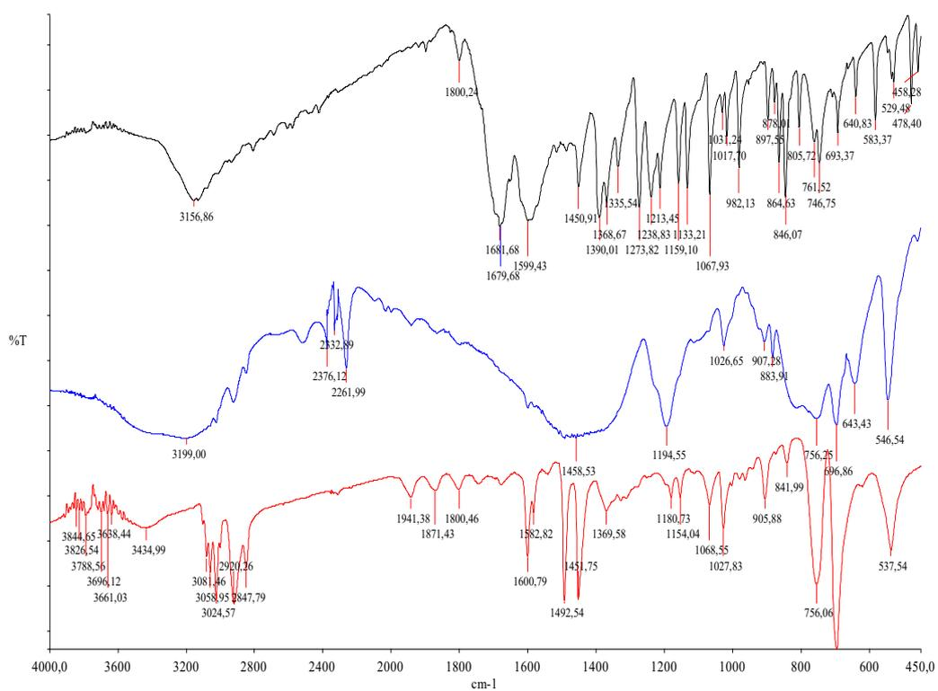
**Figure 2.** FTIR spectra of polymeric materials: PS (red), PS-K<sub>2</sub>B<sub>4</sub>O<sub>7</sub> (blue), PS-7H4MC (black).
