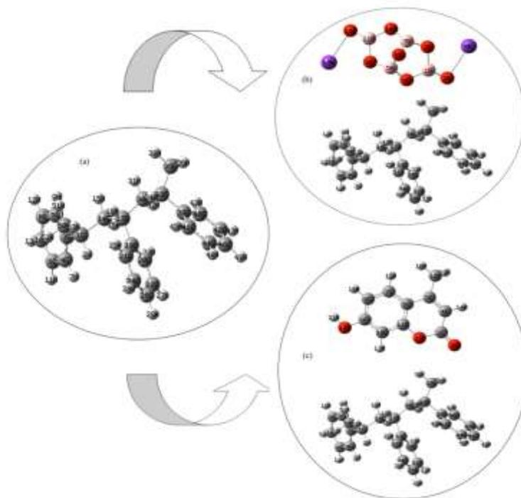
**Figure 1.** Optimized structure of polymeric materials (a) PS, (b) PS-K<sub>2</sub>B<sub>4</sub>O<sub>7</sub>, (c) PS-7H4MC.
