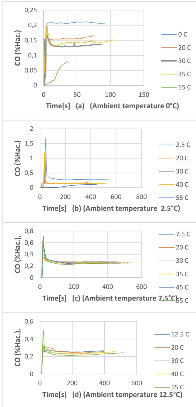
Figure 3.1 CO emission changes observed in all experiments
