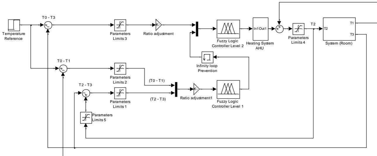
Figure 3. HVAC Controller Simulink Block Diagram
