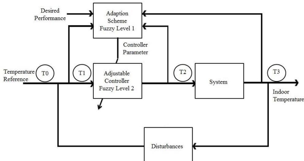
Figure 2 Controller Scheme
