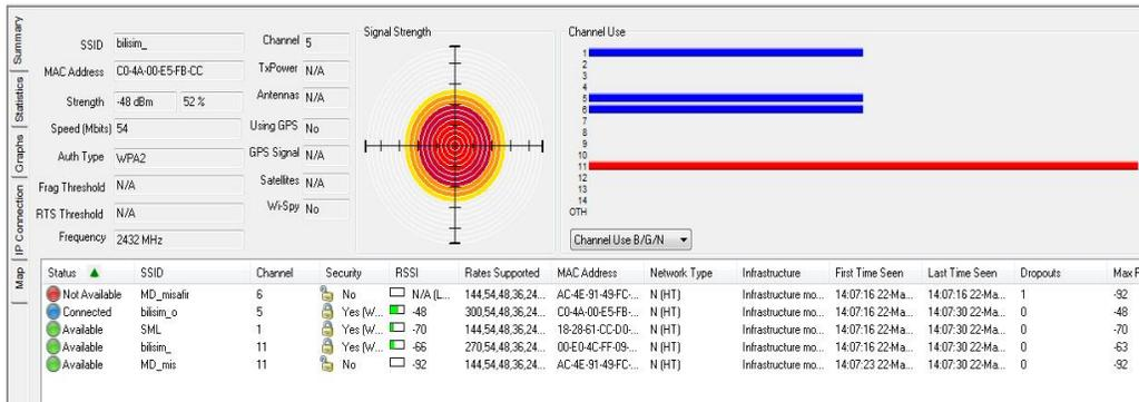
Figure 3. The channels where wireless access points have been used
