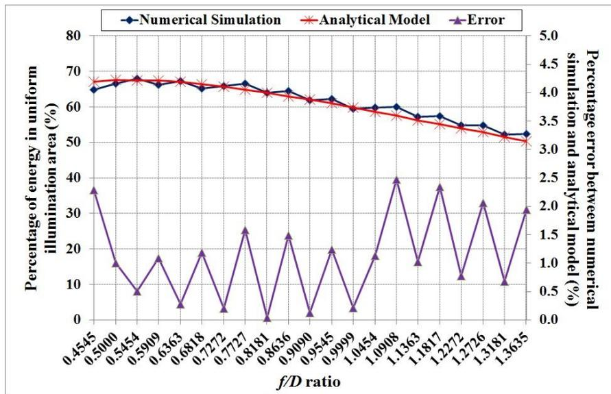
**Figure 6.** Graph shows both the percentage of energy in uniform illumination area and the percentage error between numerical simulation and analytical model versus  $f/D$  ratio.
