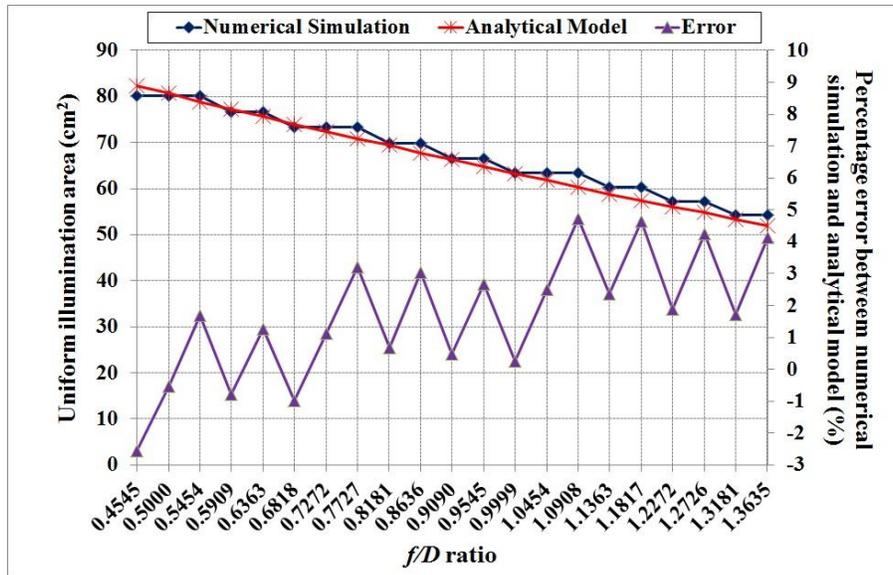
Figure 4. Graph shows both the uniform illumination area and the percentage error between numerical simulation and analytical model versus  $f/D$  ratio.
