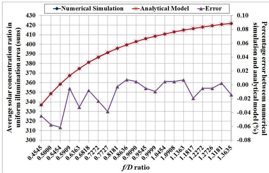
Figure 5. Graph shows both the average solar concentration ratio in uniform illumination area and the percentage error between numerical simulation and analytical model versus  $f/D$  ratio.
