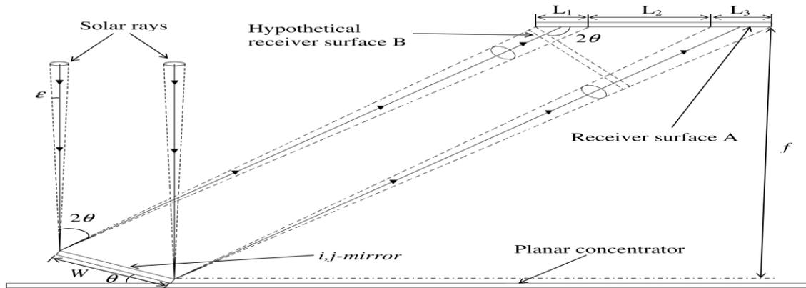
Figure 3. Cross-section view of the planar concentrator shows how the individual mirror with a dimension  $W \times W$  directs the sunlight to the receiver.
