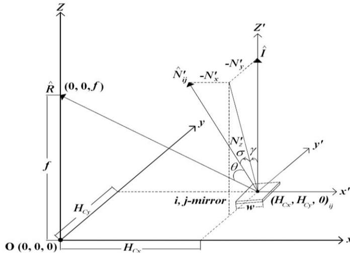
Figure 2. Cartesian coordinate system used to represent the main coordinate system  $(x, y, z)$  at the plane of the planar concentrator and the sub-coordinate system  $(x', y', z')$  is defined at the local facet mirror.
