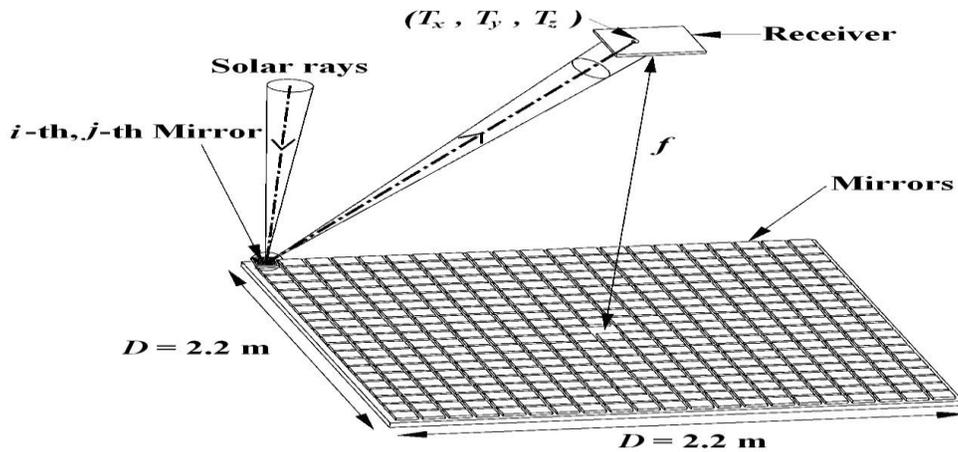
Figure 1. Conceptual layout design of the Non-Imaging Planar Concentrator (NIPC).
