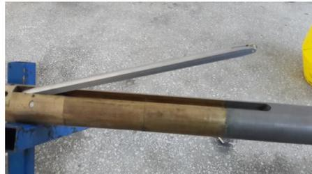
Figure 2. Opening of a caliper during density logging
