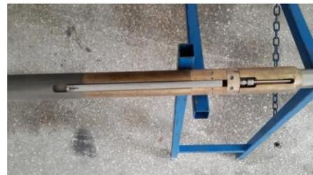
Figure 1. Single-arm caliper portion of a density log that is used for diameter measurements
