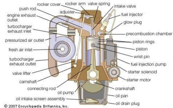
Figure 1. Diesel engine
