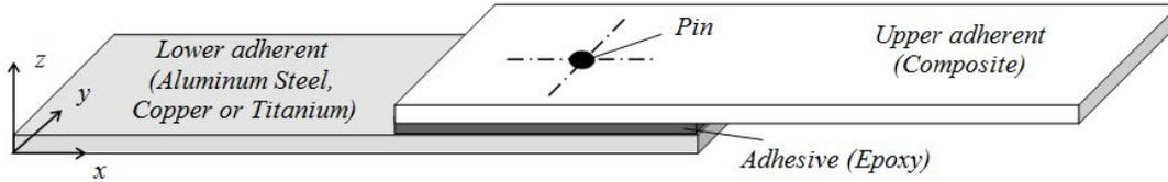
FIGURE 1. Illustration of the hybrid joint.
