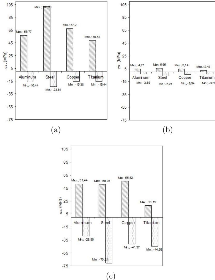
FIGURE 5. Maximum shear stresses on the hybrid joint.
