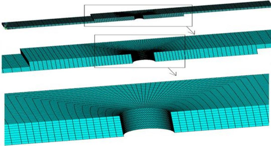
FIGURE 3. FEM structure of hybrid joint with details.
