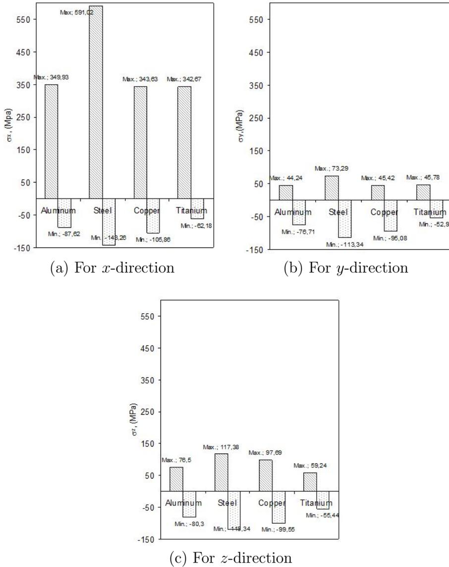
FIGURE 4. Maximum normal stresses on the hybrid joint.
