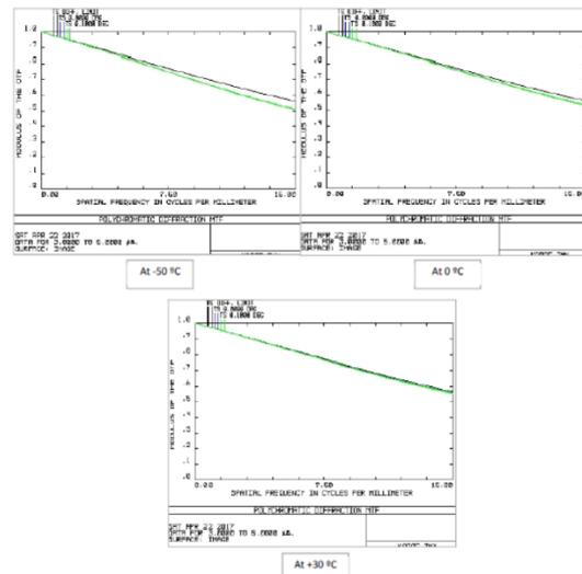
Figure 3. MTF curve diagrams for different field of view and temperature.
