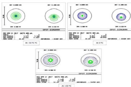
Figure 2. Spot diagrams for different field of view and temperature.
