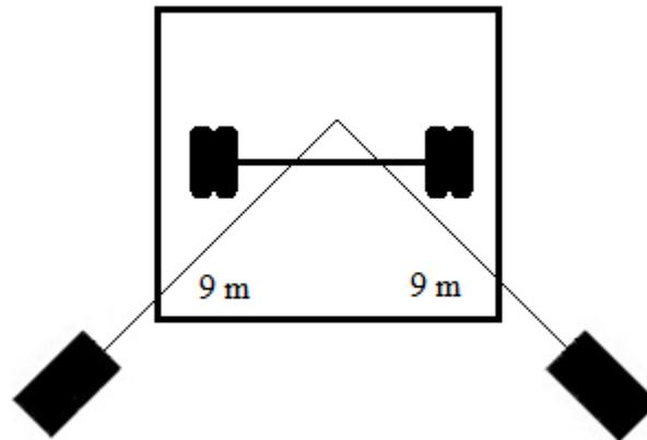
**Figure 1.** The view from the top of the camera set-up and the platform.
