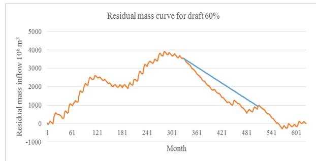
**Figure 5.** Residual mass curve method for determining the storage capacity of a reservoir with draft 60%.
