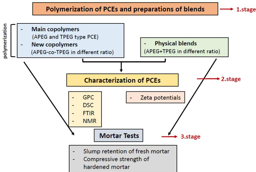
**Figure 1.** The schematic representation of the synthesis PCEs, characterization and mortar tests of PCEs
