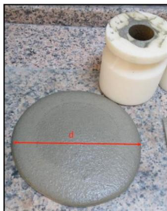
**Figure 3.** The spread flow test of mortar
