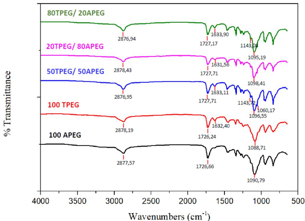
**Figure 4.** FTIR spectra for polycarboxylates
