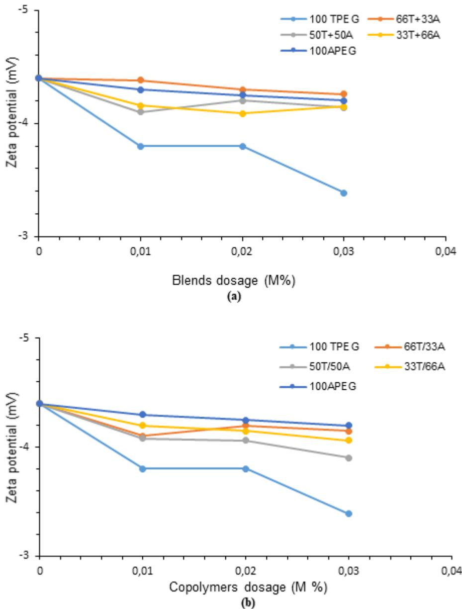
**Figure 9.** Zeta potential of cement paste with respect to a.) Blends, b.) Copolymers
