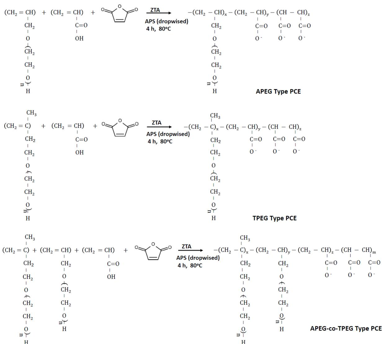
**Figure 2.** Synthesis reaction of polycarboxylate copolymers
