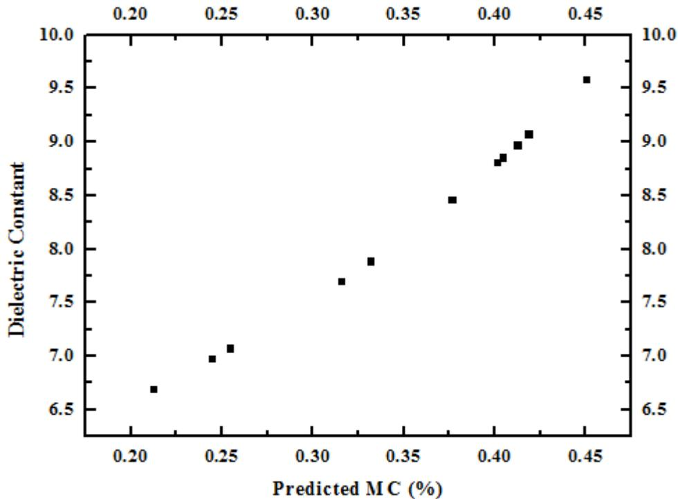
**Figure 5.** Variation of dielectric constant with predicted percentage MC
