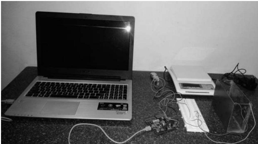
**Figure 4.** The arrangement to measure the moisture content of paddy. 1. Personal Computer 2. Bread-Board 3. Evaluation Board 4. Parallel Plate Sensor 5. Electronic Balance
