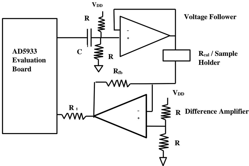
Figure 1. Circuit Diagram to measure the capacitance value
