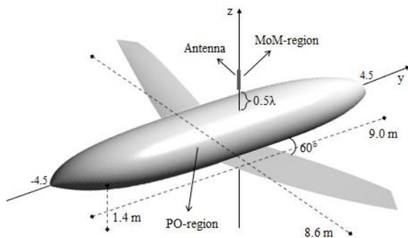
**Figure 6.** MoM and PO-region distribution for aerial vehicle example
