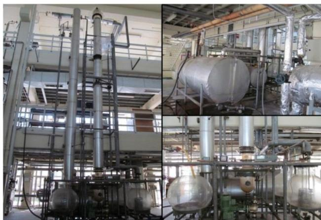
Figure 2. Pilot size distillation column.
