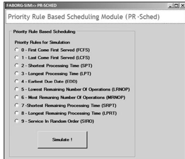
Figure 4. Priority rules in simulation module of Faborg-Sim
