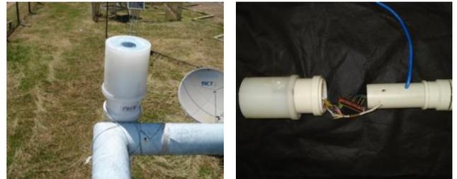
Figure 6. Assembly of the pyranometer beside a photodiode sensor (Campbell Scientific Inc., model LI200X) for comparison of the signals.
