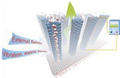
**Figure 5** Schematic illustration showing energy harvesting and conversion of the pumping system. The green arrow indicates the direction of water flow through the vibrating nanotubes
