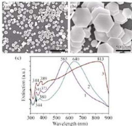
**Figure 2** FESEM images of Ag HNPs with different edge lengths: (a) 40 nm; (b) 60–350 nm; (c) UV-vis spectra of Ag HNPs where curves 1, 2, and 3 correspond to nanoplates with edge lengths of 40, 60 and 60–350 nm
